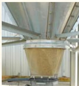
Single unloader shown with optional swing away bottom for 100% clean out.
